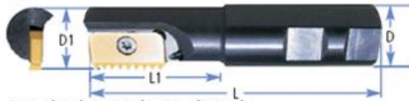
Standard Straight Neck Style (For parallel thread applications.)
